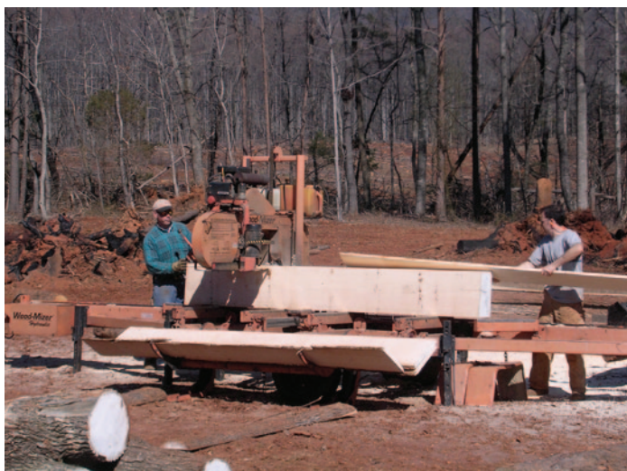
Above left, a board is sawn from a log on the author's farm with a portable sawmill. Above right, a closeup of the blade running horizontally, cutting a board from the top of the log. All images courtesy of Mark Lieberth.
