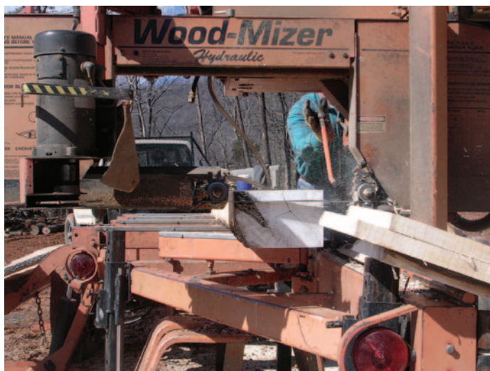
Above left, a board is sawn from a log on the author's farm with a portable sawmill. Above right, a closeup of the blade running horizontally, cutting a board from the top of the log. All images courtesy of Mark Lieberth.
