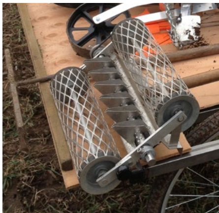
(Left) You can see the underside of a Johnny's six row seeder above, and even larger seeders would look similar from below. (Right) The Johnny's 4 row seeder is one of the simplest and smallest seeders making it good in tight spaces. Unlike most other hand scale seeders it is designed to be pulled rather than pushed. All images courtesy of the author.
