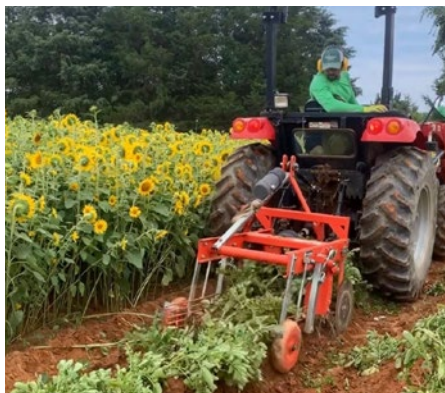
Ross Mickens of Open Door Farm in Cedar Grove, North Carolina, using the Tool Legit co-op's Checchi & Magli potato digger. Photo by Jillian Mickens.
